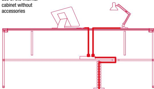
cablе scheme and use of the accessories inside the internal cabinet
